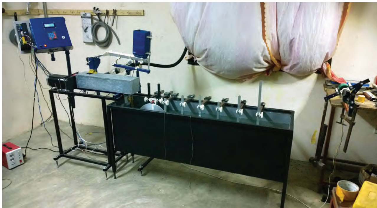
FIGURE 2 Thunderhead filament extruder prototype at STICLab in Dar es Salaam, Tanzania.
